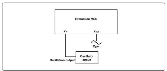
Figure 3.2 External oscillator circuit
